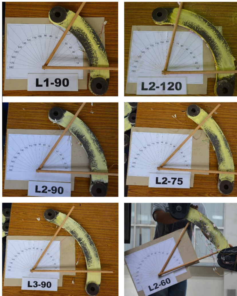
Fig. 11. Yield regions of dampers with various geometries.
