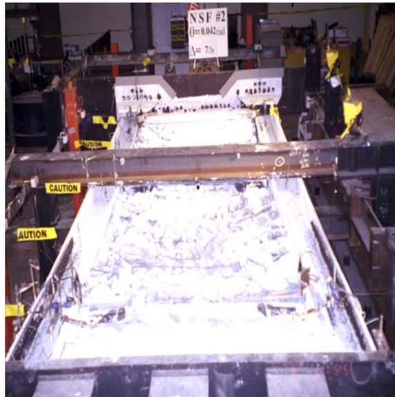
Crushing of Concrete Wall
